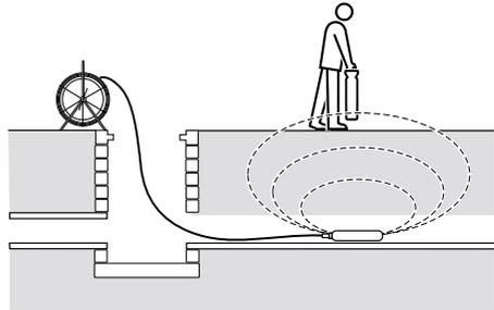
A new battery or a freshly recharged battery should be used at the beginning of each day and preferably at the start of a job. Check that the locator and sonde are working correctly.
