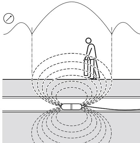
With the locator sensitivity set as desired, propel the sonde along three to four paces and stop.
